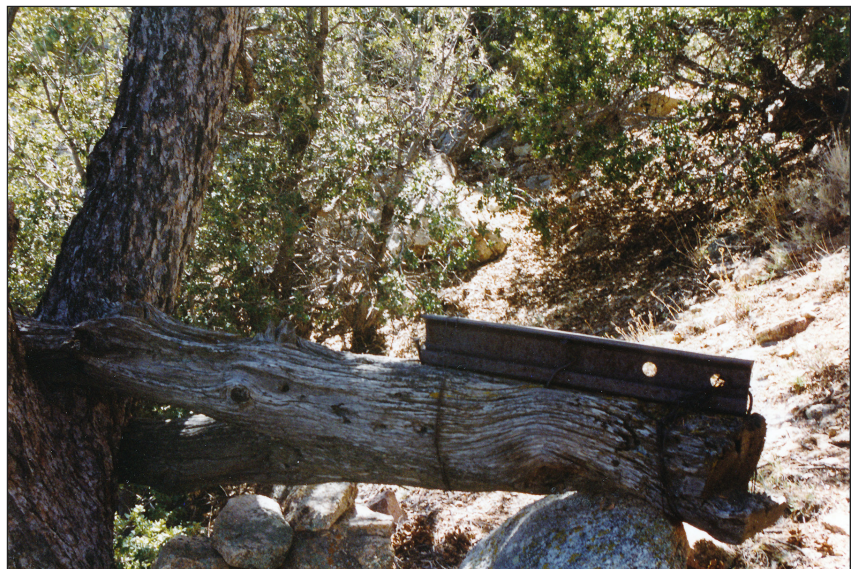
Figure 3. Anvil made of railroad track, wired to forked log and braced by tree and rock, at the New York Peak prospect, 1994. R.E. Reynolds photograph.
