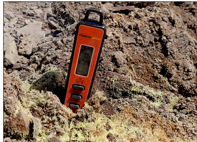
Figure 9. Vent showing yellow acicular sulfur crystals. Temperature 10 cm below surface was 440°C (824°F).
